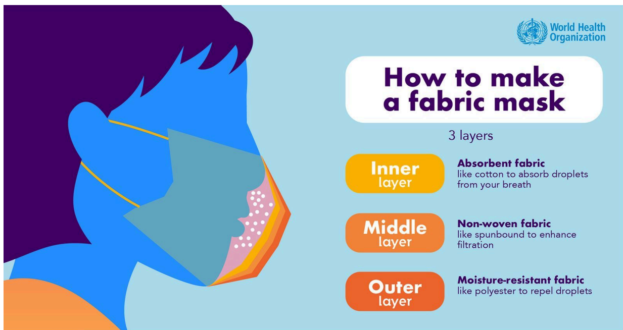
Figure 1. Non-medical mask construction using breathable fabrics such as cotton, cotton blends, polyesters, nylon and polypropylene spunbond that are breathable may impart adequate filtration performance when layered. Single- or double-layer combinations of advanced materials may be used if they meet performance requirements [9]
